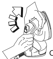
C Turn the soleplate clockwise using the specific handle
