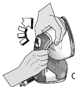
C Turn the soleplate clockwise using the specific handle
