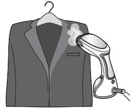
Pull the fabric taut with your free hand. Applying slight pressure, put the appliance on the spot that is creased. Briefly press the steam jet button and then release it.
