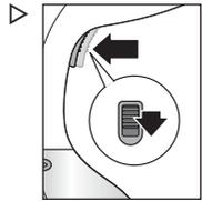
To release steam continuously, you can lock the steam jet button in place.
