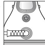
The indicator light flashes while the appliance is heating up. Once the indicator light stays lit, the operating temperature has been reached.
