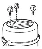
To help get the wheels into the sockets first smear a little washing up liquid onto the plastic wheel shaft threads. Then place a metal rod (use a large screwdriver, sharpening steel or heavy spoon handle etc.) between the two wheels. Wrap your fingers around the wheels and grasp the rod in the palm of the hand so that you can exert pressure evenly on the metal bar thus driving the main force directly through the wheel shaft.
