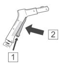
To start the steam push the red safety locking button [1] underneath the handle forward then squeeze the trigger [2] and steam will start to flow. It is normal for a few drops of water to come out first.
