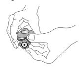
b Make sure black neoprene washer is in place on the regulator iniet. Regularly examine, and if unduly compressed or damaged, replace. Do not replace with red branch cap washer.
