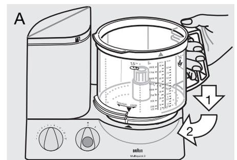
2. Put the attachment needed (see instructions for each of the attachments) onto the drive shaft of the bowl and push it down as far as it will go.
