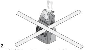
DO NOT place clothes or other materials on the Heater, as apart from the danger of fire their presence could affect the efficient working of the appliance.
