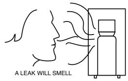
IF a leak is suspected, turn the gas off at cilinder. DO NOT disconnect the regulator. Extinguish all naked lights. Check all connections. Slowly turn the gas on a brush the connectors with soapy water or liquid detergent - a gas leak will form bubbles. If a leak is found turn the gas off and inform your Dealer. DO NOT use the heater again until it has been inspected by your Dealer.
