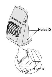
3) Fit the front panel assembly to the base plate by fixing the two screws (removed previously) trough the aligned screw holes (holes D and A).
