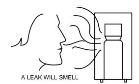
IF a leak is suspected, turn the gas off at cilinder. DO NOT disconnect the regulator. Extinguish all naked ligh Check all connections. Slowly turn the gas on a brush connectors with soapy water or liquid detergent - a gas leak will form bubbles. If a leak is found turn the gas o and inform your Dealer. DO NOT use the heater again until it has been inspected by your Dealer.
