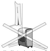
DO NOT position Heater alongside a wall or near curtains, etc. ALWAYS face Heater towards centre of room.
