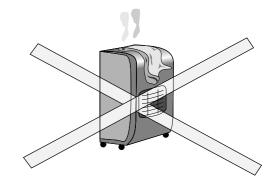
DO NOT place clothes or other materials on the Heate as apart from the danger of fire their presence could affect the efficient working of the appliance.
