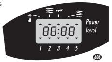
Press the **function** button to select combination microwave and grill cooking. The display will flash "0:00" and the micro & grill indicator will light.
