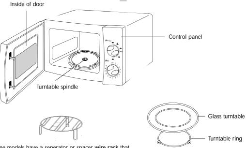
Some models have a seperator or spacer wire rack that makes it possible to cook two food dishes at the same time (simultaneous insertion of two plates or pans).
