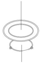
Wash the rotating ring in warm water. Don't use very hot water which could make it warp.
