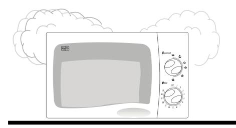
Your microwave is designed to let steam escape from the vents and around the door without microwave energy escaping.
