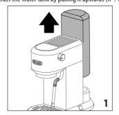
Open the water tank lid (A1) and fill the water tank (A2) with fresh clean water, taking care not to exceed the MAX level (fi . 2).
