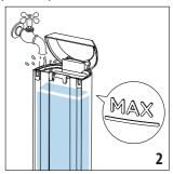
**Please note:** Never operate the appliance without water in the water tank or without the tank.
