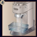
Place a container with a minimum capacity of 500 ml under the coffee outlet and steam wand .
