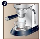
Attach the portafilter to the machine and place the cup under the portafilter spouts.
