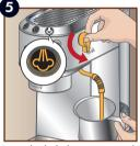
Once the light becomes steady, place the recipient containing the milk under the steam wand: immerse the frother and open the steam dial.
