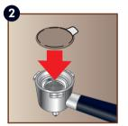
Insert the pod, centring it as far as possible on the filter.
