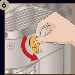
Turn the hot water/steam dial to the position and deliver to empty the water tank; then turn the knob to the 0 position. This is to purge the steam circuit before frothing or steaming your milk.
