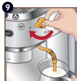
Once the desired temperature is reached turn the steam knob off and wait till steam stops completely before removing jug.
