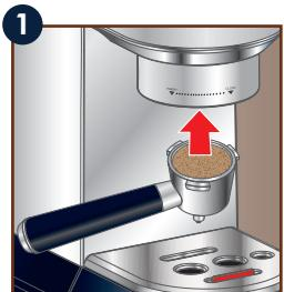
Remove any excess coffee from the rim of the portafilter and attach the portafilter to the machine.
