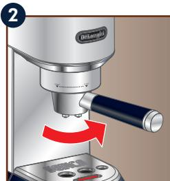
Lock the portafilter securely in the brewing unit rotating it to the right..
