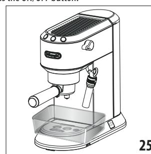
3. Make sure the filter holder is not attached and position a recipient under the hot water spout and coffee outlet (A5) (fig. 25).
