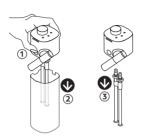
2 Position the milk spout vertically to disassemble and to reassemble.
