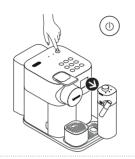
2 Remove the water tank. Lift and close the lever to eject any remaining capsule. Place a container under the coffee outlet.
