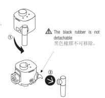
Turn the Rapid Cappuccino System connector until the "unlock △" symbol and extract it.
