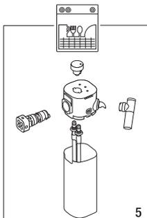
**i** In case a dishwasher is not available, refer to section «Hand washing of Rapid Cappuccino System» of the user manual. In the case the milk container is kept outside refrigerator for longer than 30 min, disassemble the Rapid Cappuccino System and clean all components
