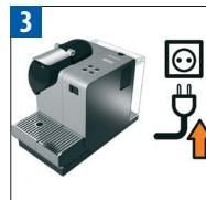
Put the machine in the upright position and plug it into the mains.
