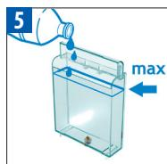
Rinse the water tank before filling with potable water up to the maximum level.
