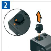
Remove the milk froth regulator knob by turning it to (►) and pulling it up.
