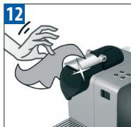
Clean the machine using a damp cloth. You have now finished descaling the machine.
