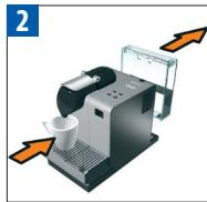
Remove the water tank. Close the lever (without a capsule inside). Place a container under the coffee outlet.
