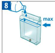
Empty the used capsule container and drip tray, rinse and fill the water tank with fresh potable water up to the MAX level. Repeat step 5 again.
