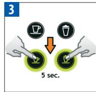
Press the Cappuccino and Espresso buttons simultaneously for 5 seconds. Preparation buttons blink alternately: emptying mode is in progress.
