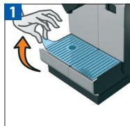
Remove the plastic film from both the left and right grid, and machine panels.
