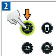
Press and hold the Espresso or Lungo button. Brewing starts. Button blinks quickly: programming mode.
