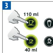
Press the Espresso (40 ml) or the Lungo (110 ml) button. Preparation will stop automatically. To stop the coffee flow or top up your coffee, press again.
