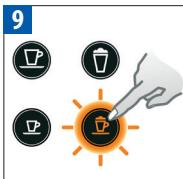
Press the Cappuccino button again. The rinsing cycle continues through the coffee outlet, descaling pipe and drip tray until the water tank is empty.
