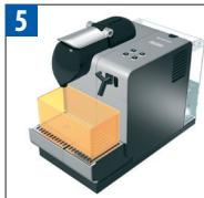
Place a minimum 1 litre container under both the coffee outlet and descaling pipe nozzle.
