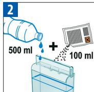
Empty the drip tray and the used capsule container. Fill the water tank with 100 ml of Nespresso descaling agent and 500 ml water.
