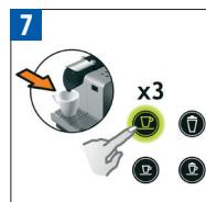
Rinsing: place a container under the coffee outlet and press the Lungo button. Repeat three times.
