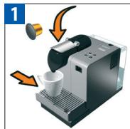
Fill the water tank, switch the machine on and insert the capsule. Close the lever and place a cup under the coffee outlet.
