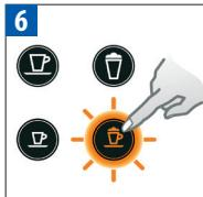
Press the Cappuccino button. The descaling agent flows alternately through the coffee outlet, descaling pipe and drip tray. The Cappuccino and Macchiato button blink alternatively.
