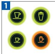
Descale the machine when the Cappuccino button shines orange in ready mode (descaling alert).
