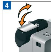
Take the cup. Lift and close the lever to eject the capsule into the used capsule container.
