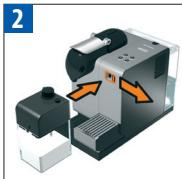
Close the milk container. Open the steam connector door by sliding it to the right.
