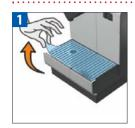
Remove the plastic film from both the left and right grid, and machine panels. 移除左右滴水柵格及咖啡機 兩旁的之膠片。
