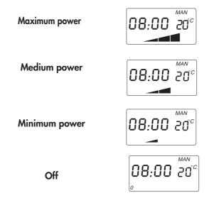
If Maximum power has been selected, press the " & +" or " & -" button to select the desired comfort temperature from 5 to 35°C. By pressing the " & +" or " & -" button the desired temperature (shown on the right side of the display) will increase or decrease by 1°C. Keep pushbutton pressed to move through the temperature in fast mode.
