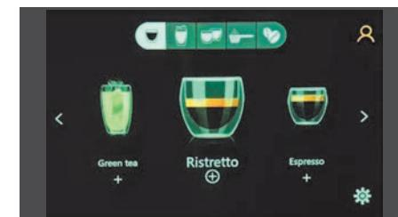
Press the BEVERAGE PARAMETERS button (+) to access the relevant beverage parameters.
