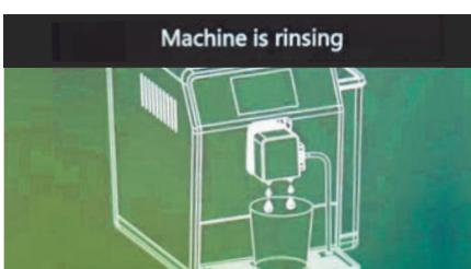
The appliance starts the rinsing stage of the internal circuits and waste water is dispensed from the coffee dispensing spout. The display of the appliance shows the appropriate screen.
