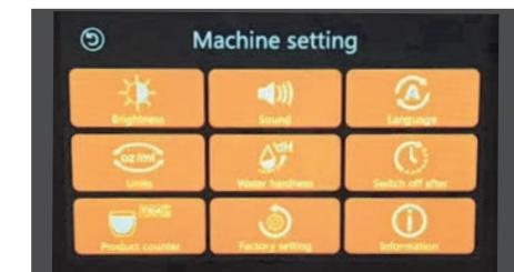
When using the appliance for the first time or after resetting to factory settings, the appliance language, unit of measurement and water hardness must be set up.
