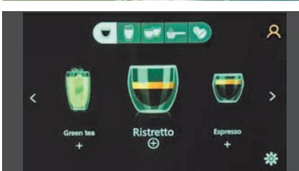
After the heating phase and the internal circuit rinsing stage, the initial screen is displayed and the appliance is ready to be used.
