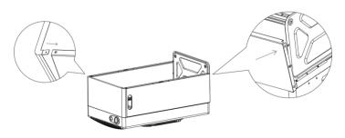
3 Fix two wheels directly to the bottom of (E) the front panel and fix 2 wheels with the (C) bottom plate with the 2 nuts provided (M8). Use 4 screws (M5x8) to fix the bottom plate with the left and right-side panel. Fix the corner panel with side panels by 2 screws (ST4x8).
