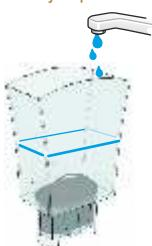
Tilt the water tank back and forth to remove air bubbles from the filter.
