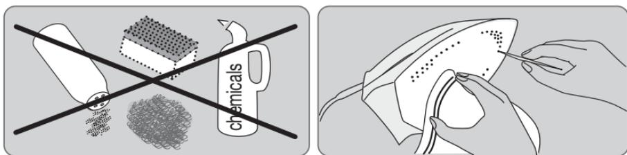
**F** Cleaning the anti-calc valve
