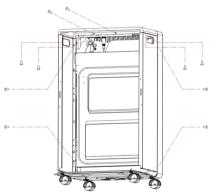
5 Put the (F) back panel on two side panels after you place the gas cylinder on the bottom plate.
