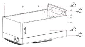
4 Fix the (D) top panel with (E) the front panel by 2 screws (ST4x8). Use 4 screws (ST4x8) to fix the top panel with left and right panel. Fix the left and right panel with the front panel with the 4 screws (ST4x8).
