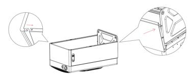
3 Fix two wheels directly to the bottom of (E) the front panel and fix 2 wheels with the (C) bottom plate with the 2 nuts provided (M8). Use 4 screws (M5x8) to fix the bottom plate with the left and right-side panel. Fix the corner panel with side panels by 2 screws (ST4x8).
