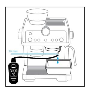
The optimal indicative temperature measurement for hot water should be 93°C±2°C.
