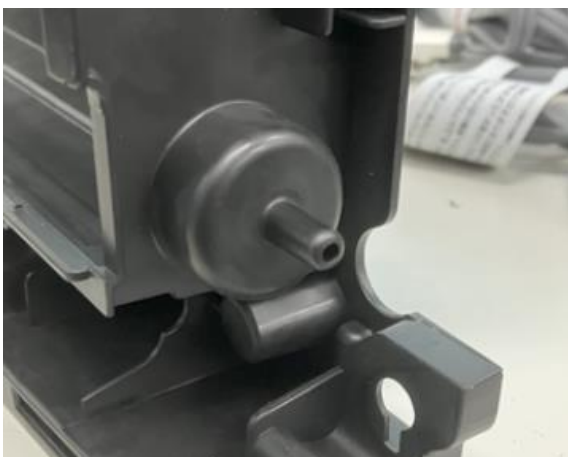
Chassis with embedded water tube.
